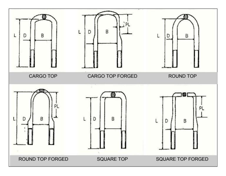
U/Bolts can be made to order - given the specifications supplied
